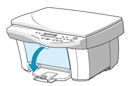
3 Locate the print cartridge holder inside the product. The black ink cartridge holder is located on the right side of the cartridge holder and the colour ink cartridge is located on the left side.
